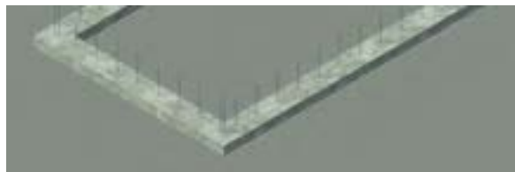
Strip footing with vertical rebar inplace.
